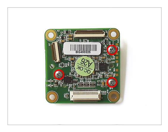
• Place the lens holder over the sensor on the front of the PCB. Turn the PCB over. Using the two fixing screws provided, affix the lens holder from the back of the PCB. The red circles above show the placement of the fixing screws.
