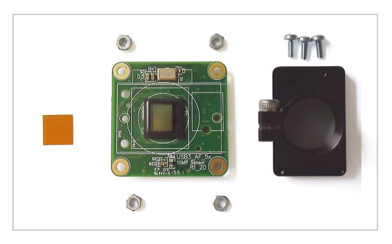
• Remove protective foil from sensor
