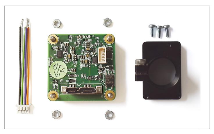
• Unscrew the four nuts from the camera back.
