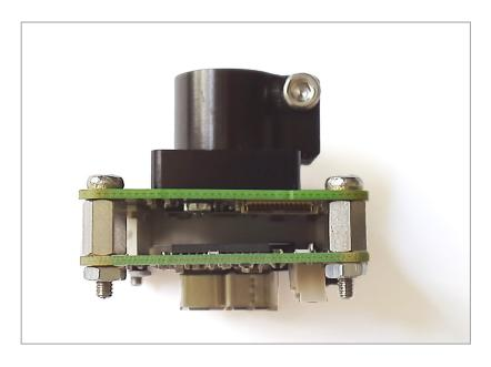
With the lens holder now mounted to the front of the PCB, replace the back PCB to its original position ensuring that the inter PCB connector is closed.
