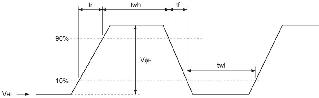
**(4) Reset gate clock waveform**
