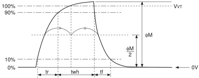
(2) Vertical transfer clock waveform
