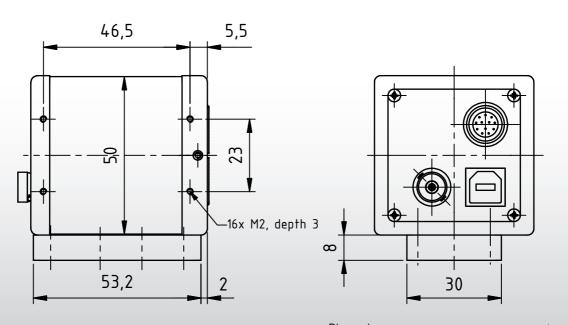
Dimensions: mm Tolerances: DIN ISO 2768m
