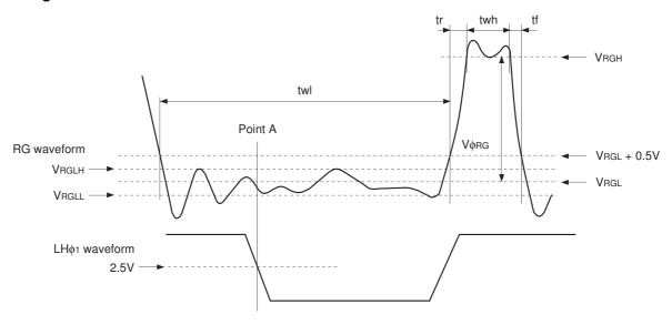
VRGLH is the maximum value and VRGLL is the minimum value of the coupling waveform during the period from Point A in the above diagram until the rising edge of RG.
