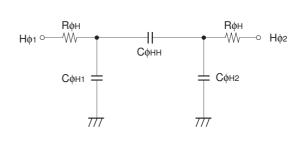
Vertical transfer clock equivalent circuit
