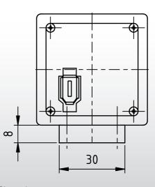
Dimensions: mm Tolerances: DIN ISO 2768m
