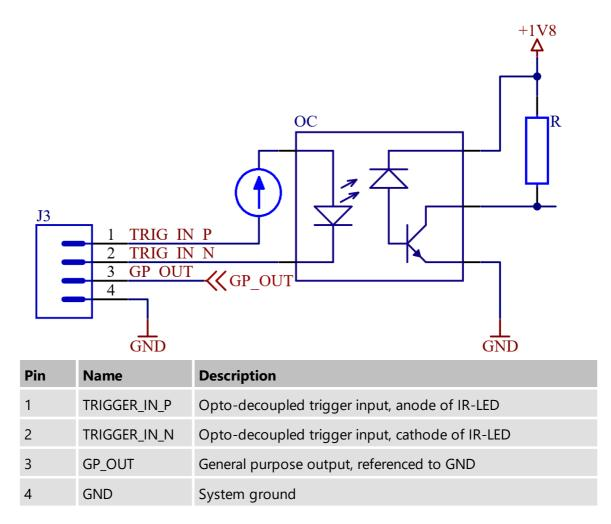
The trigger input is opto-decoupled. To drive the trigger input, a voltage must be applied to pins 1 and 2. Note: pin 1 is the positive input; pin 2 is the negative input.
