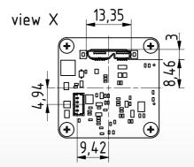
Dimensions: mm Tolerances: DIN ISO 2768m
