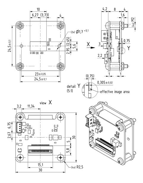
Scale: 2:1 Dimensions: mm Tolerances: DIN ISO 2768-m
