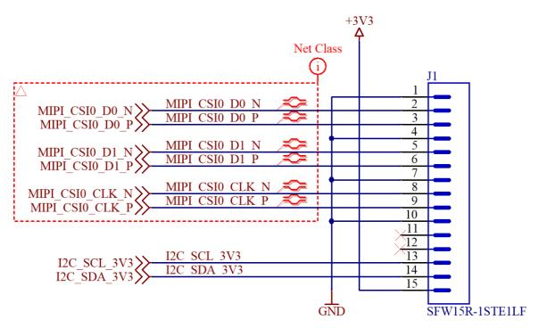
The I2C-bus signals have the I/O voltage of 3.3V.
