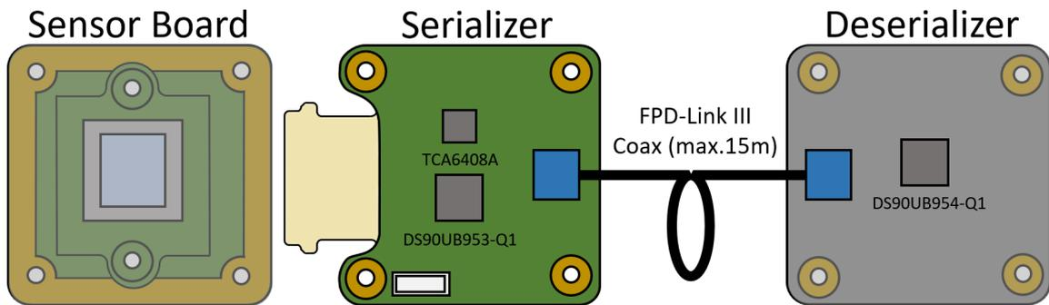
The document "Deserializer Design Recommendations" contains important information required to create a custom deserializer design using the TI DS90UB954-Q1 chip.
