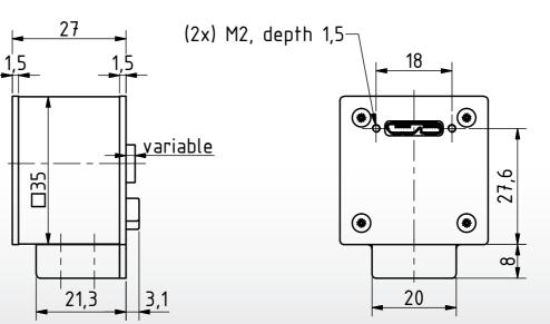
Dimensions: mm Tolerances: DIN ISO 2768m
