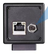
PWR: please put 1: and 2: together and feed the camera with 12VDC/1A to 24VDC/0.5A.
