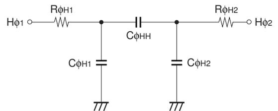
**Horizontal transfer clock equivalent circuit**
