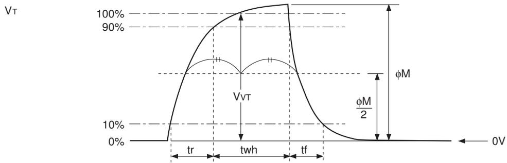
Note) Readout clock is used by composing vertical transfer clocks  $V\phi_2$  and  $V\phi_3$ .
