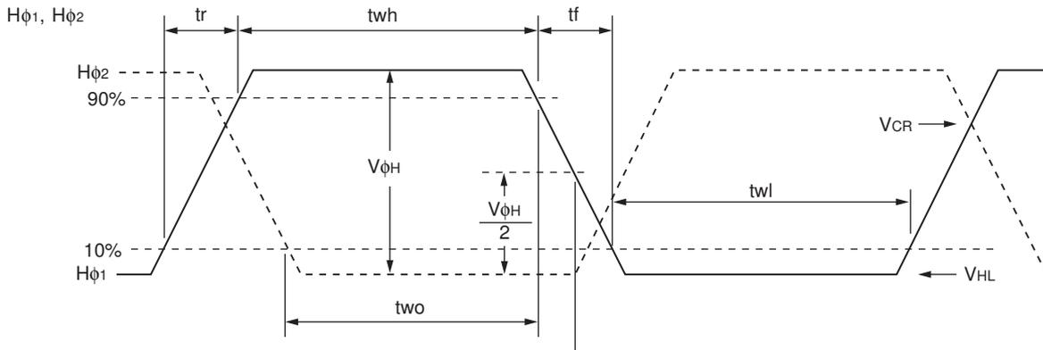
Cross-point voltage for the Hφ1 rising side of the horizontal transfer clocks Hφ1 and Hφ2 waveforms is V<sub>CR</sub>. The overlap period for t<sub>wh</sub> and t<sub>wl</sub> of horizontal transfer clocks Hφ1 and Hφ2 is two.
