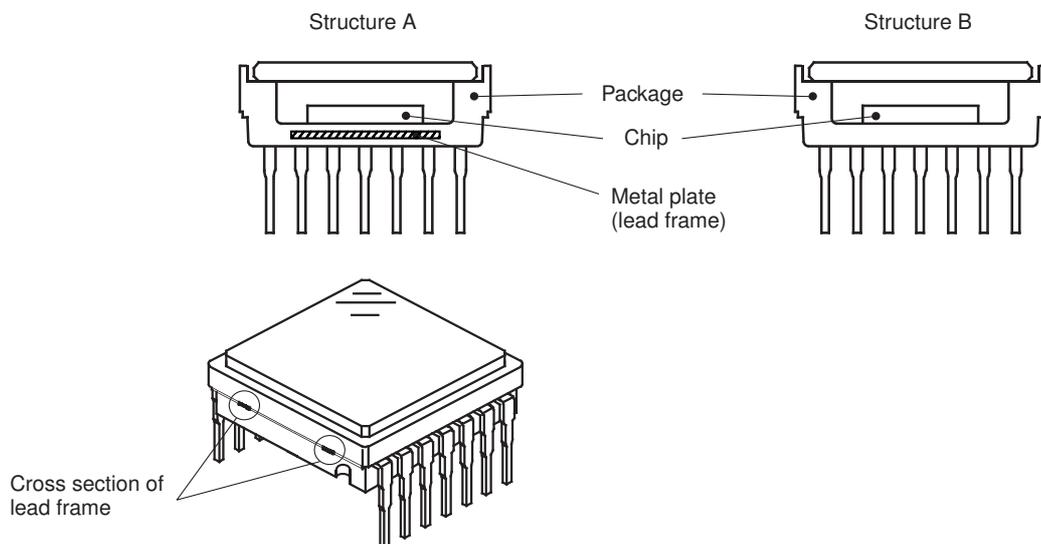
The cross section of lead frame can be seen on the side of package for structure A.
