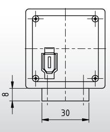
Dimensions: mm Tolerances: DIN ISO 2768m
