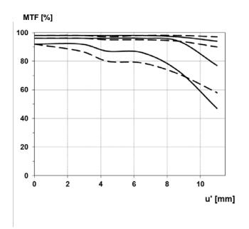
The Modulation Transfer (MTF) as a function of image height (u) and slit orientation (sagittal, tangential) has been measured with white light at spatial frequencies of R = 10, 20 and 40 cycles/mm.
