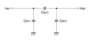
Vertical transfer clock equivalent circuit
