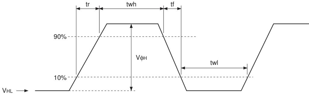
**(4) Reset gate clock waveform**
