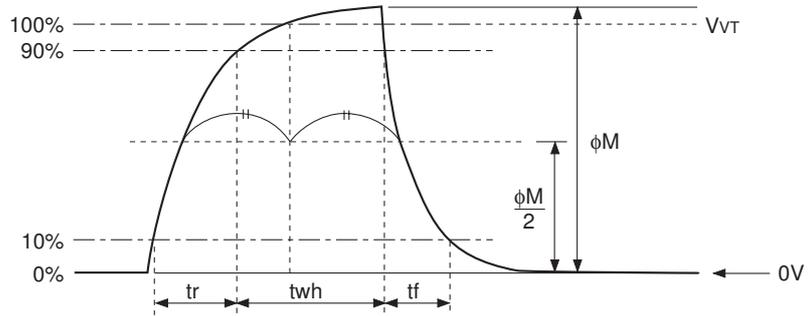
(2) Vertical transfer clock waveform
