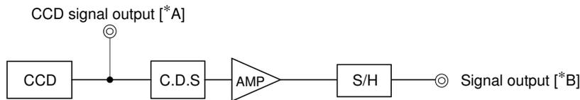
**Note)** Adjust the amplifier gain so that the gain between [\*A] and [\*B] equals 1.
