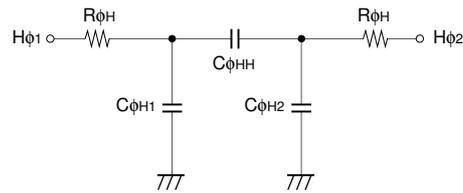
**Horizontal transfer clock equivalent circuit**
