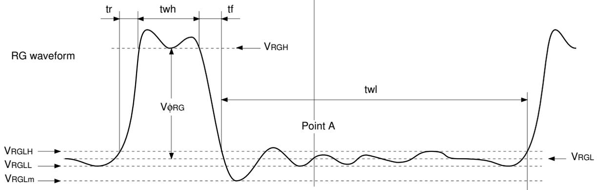
VRGLH is the maximum value and VRGLL is the minimum value of the coupling waveform during the period from Point A in the above diagram until the rising edge of RG. In addition, VRGL is the average value of VRGLH and VRGLL.
