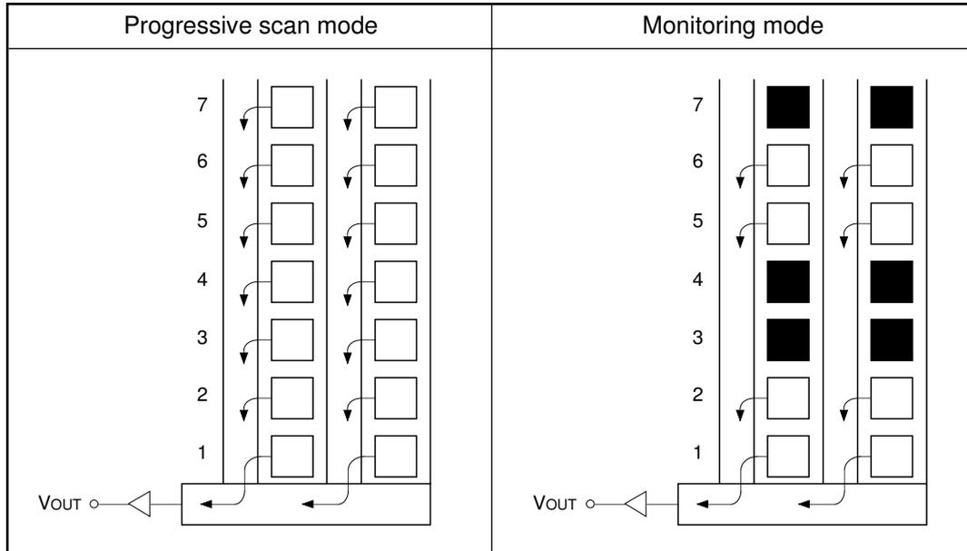
**Note)** Blacked out portions in the diagram indicate pixels which are not read out.
