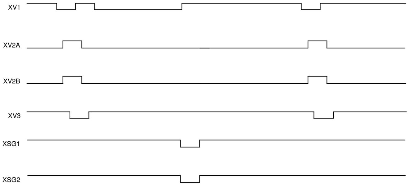
Sensor readout clocks XSG1 and XSG2 are used by composing XV2A and XV2B.
