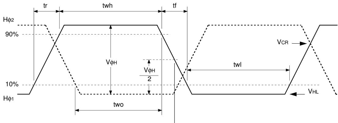
Cross-point voltage for the Hφ1 rising side of the horizontal transfer clocks Hφ1 and Hφ2 waveforms is VCR. The overlap period for twh and twl of horizontal transfer clocks Hφ1 and Hφ2 is two.
