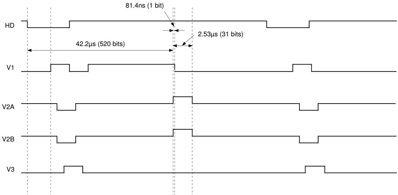
Sensor Readout Clock Timing Chart      Monitoring Mode
