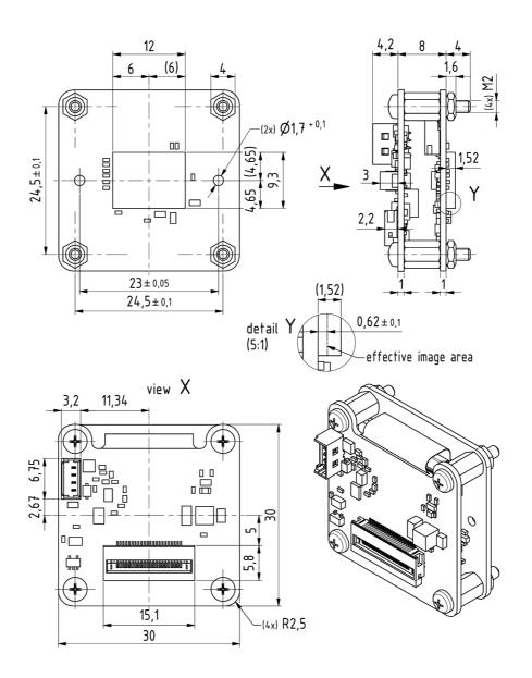
Scale: 2 : 1 Dimensions: mm Tolerances: DIN ISO 2768-m 289-20-6-06-00
