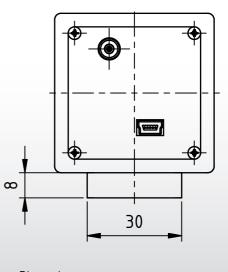
Dimensions: mm  $\Box \oplus$ Tolerances: DIN ISO 2768m
