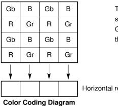
The primary color filters of this image sensor are arranged in the layout shown in the figure on the left (Bayer arrangement). Gr and Gb denote the G signals on the same line as the R signal and the B signal, respectively.
