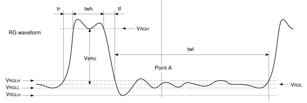
VRGLH is the maximum value and VRGLL is the minimum value of the coupling waveform during the period from Point A in the above diagram until the rising edge of RG.
