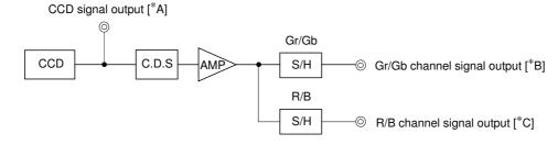
Note) Adjust the amplifier gain so that the gain between [\*A] and [\*B], and between [\*A] and [\*C] equals 1.
