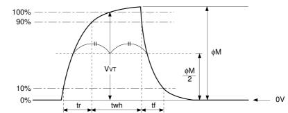
Note) Readout clock is used by composing vertical transfer clocks V<sub>\$\phi2A</sub> and V<sub>\$\phi2B</sub>.
