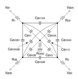
Vertical transfer clock equivalent circuit
