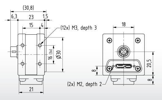
Dimensions: mm Tolerances: DIN ISO 2768m
