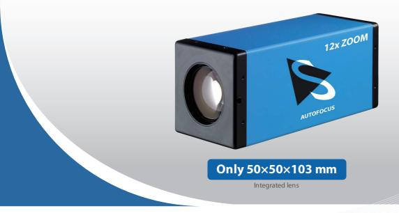
The Imaging Source DMK Z12G445 monochrome camera has a GigE interface and is the perfect solution for many industrial automation, quality assurance, security, surveillance and medical applications. The monochrome camera ships with the very sensitive 1/3 inch Sony CCD ICX445ALA sensor. With up to 30 images per second, the DMK Z12G445 is a low cost, yet highly versatile imaging solution. The camera integrates an autofocus lens (Automatic/manual)
