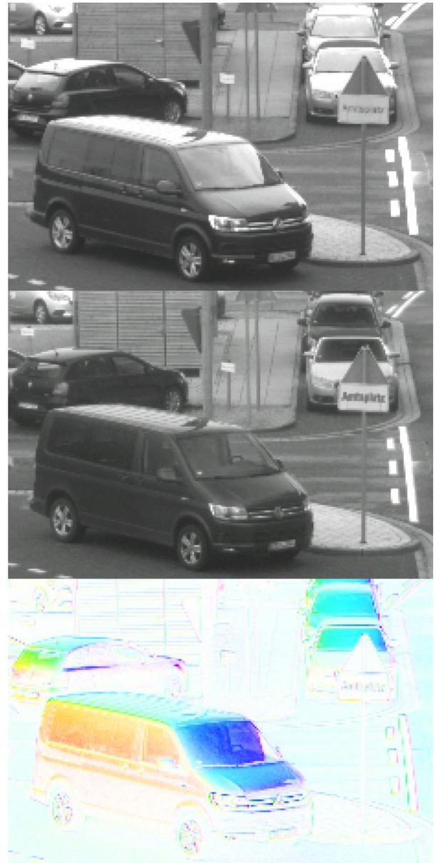
**Fig. 12:** Top image: Image from standard sensor showing heavy surface reflection.
