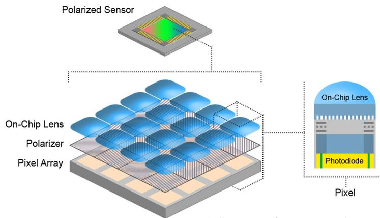
Fig. 1: Illustration of Sony's new polarization sensor
