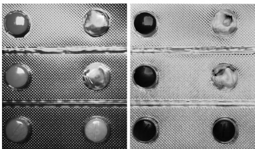
**Fig. 7 (left):** Shows a standard intensity image (left) of medication in blister pack with low contrast and glare. The right image from DZK 33UX250 (DoLP processing) shows improved contrast and significant glare reduction, making presence inspection more accurate..
