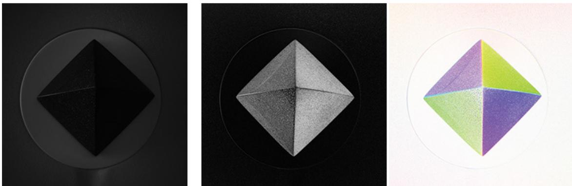
**Fig. 8** Intensity image (left) displays poor contrast overall. DoLP processing of the polarization data (middle) adds contrast; AoLP processing of the polarization data with HSV color mapping (right) from DZK 33UX250 adds additional image information which can be used for effective segmentation.
