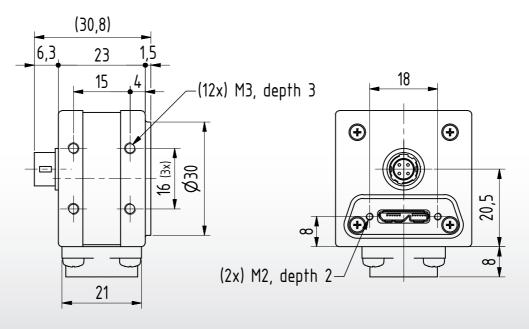
Dimensions: mm Tolerances: DIN ISO 2768m
