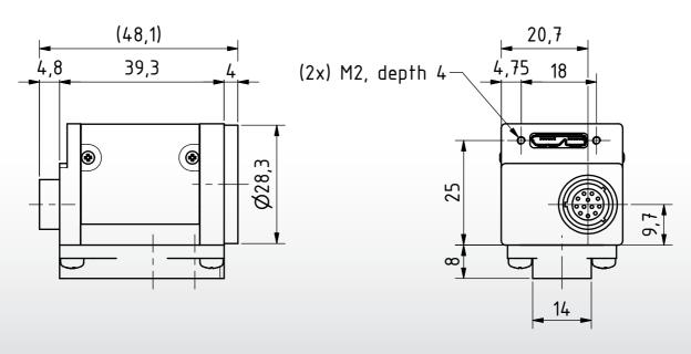
Dimensions: mm Tolerances: DIN ISO 2768m
