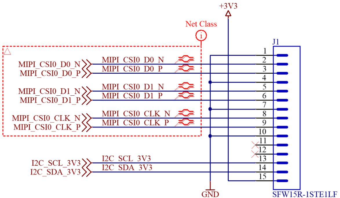
The I2C-bus signals have the I/O voltage of 3.3V.
