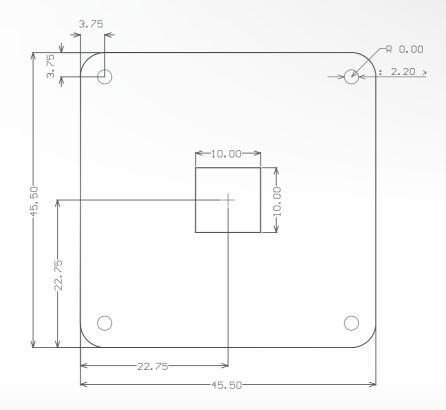
Dimensions: mm Tolerances: DIN ISO 2768m
