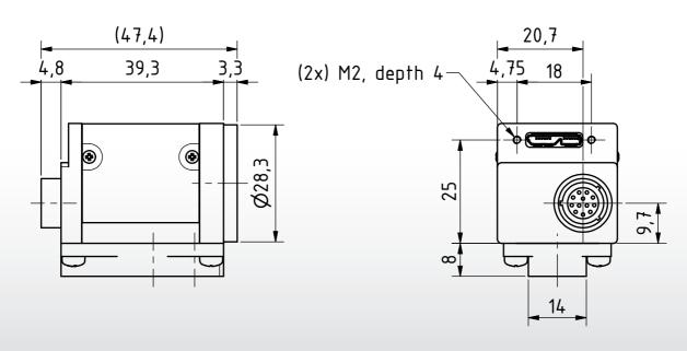
Dimensions: mm Tolerances: DIN ISO 2768m
