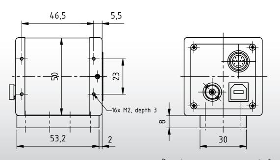
Dimensions: mm Tolerances: DIN ISO 2768m
