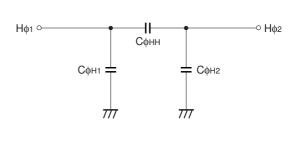
Vertical transfer clock equivalent circuit
