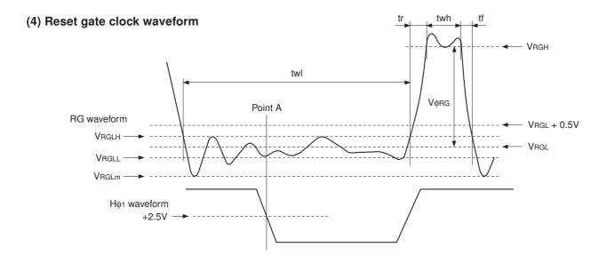
VRGLH is the maximum value and VRGLL is the minimum value of the coupling waveform during the period from Point A in the above diagram until the rising edge of RG. In addition, VRGL is the average value of VRGLH and VRGLL.
