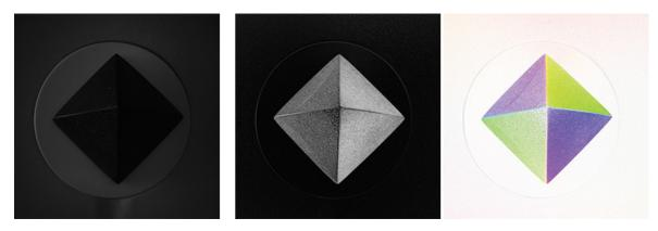
Fig. 8 Intensity image (left) displays poor contrast overall. DoLP processing of the polarization data (middle) adds contrast; AoLP processing of the polarization data with HSV color mapping (right) from DZK 33UX250 adds additional image information which can be used for effective segmentation.
