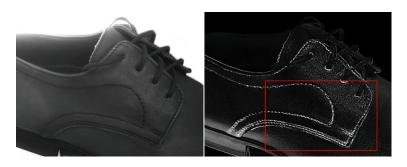
Fig. 5 (left): Left image made with standard imaging sensor. On the right, DoLP processing of the polarization data dramatically improves the contrast between the leather and stitching.
