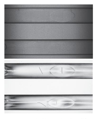
**Fig. 11**: Intensity image (top) shows little contrast, making visualization of defects difficult. Bottom image made with DZK 33UX250 using DoLP processing shows improved contrast,making scratches visible
