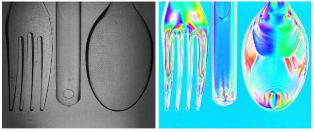
Fig. 10: Intensity image (left). Image from DZK 33UX250 (right), using AoLP processing of the polarization data and HSV colormapping to show residual stress in plastic (birefringence).
