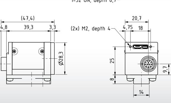
$\Box \oplus$ Dimensions: mm Tolerances: DIN ISO 2768m
