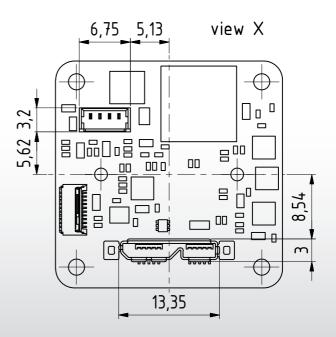
Scale: 2:1 Dimensions: mm Tolerances: DIN ISO 2768m  $\Box \oplus$
