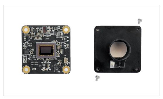
• With the orientation of the PCB and lens holder as shown in the photo, set the lens holder on top of the sensor.
