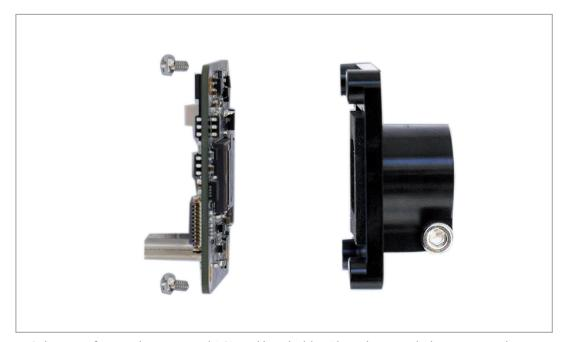
• Side view of correctly positioned PCB and lens holder. Place the provided screws into the **smaller** holes in the back of the PCB to affix the lens holder to the PCB.
