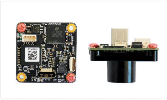
• Correct placement of provided screws shown in red. Camera is now ready for use. Remaining holes can be used to affix the camera to other hardware.
