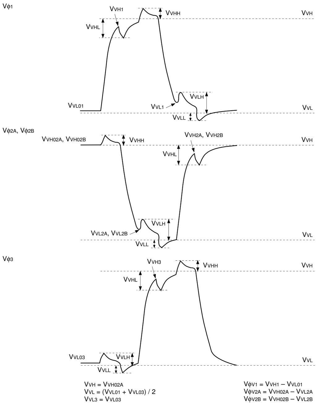
**(3) Horizontal transfer clock waveform**
