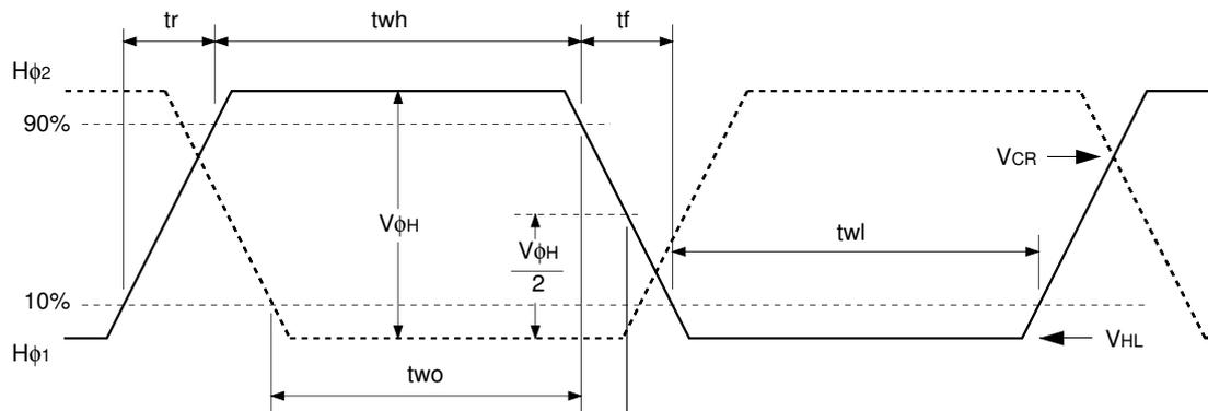
Cross-point voltage for the  $H\phi_1$  rising side of the horizontal transfer clocks  $H\phi_1$  and  $H\phi_2$  waveforms is  $V_{CR}$ . The overlap period for  $t_{wh}$  and  $t_{wl}$  of horizontal transfer clocks  $H\phi_1$  and  $H\phi_2$  is  $two$ .
