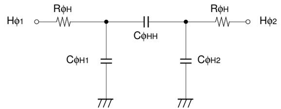
**Horizontal transfer clock equivalent circuit**
