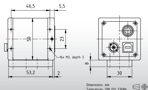
Dimensions: mm Tolerances: DIN ISO 2768m
