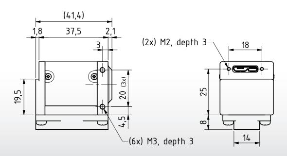
Dimensions: mm Tolerances: DIN ISO 2768m
