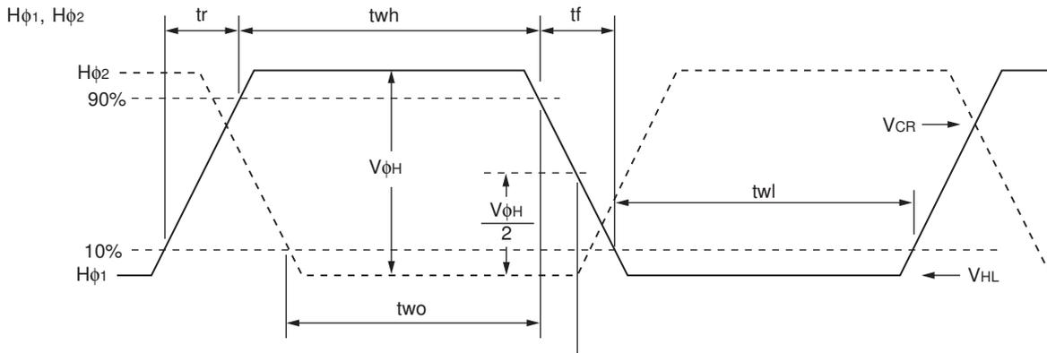
Cross-point voltage for the Hφ<sub>1</sub> rising side of the horizontal transfer clocks Hφ<sub>1</sub> and Hφ<sub>2</sub> waveforms is V<sub>CR</sub>. The overlap period for t<sub>wh</sub> and t<sub>wl</sub> of horizontal transfer clocks Hφ<sub>1</sub> and Hφ<sub>2</sub> is two.
