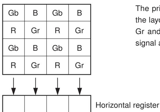
The primary color filters of this image sensor are arranged in the layout shown in the figure on the left (Bayer arrangement). Gr and Gb denote the G signals on the same line as the R signal and the B signal, respectively.
