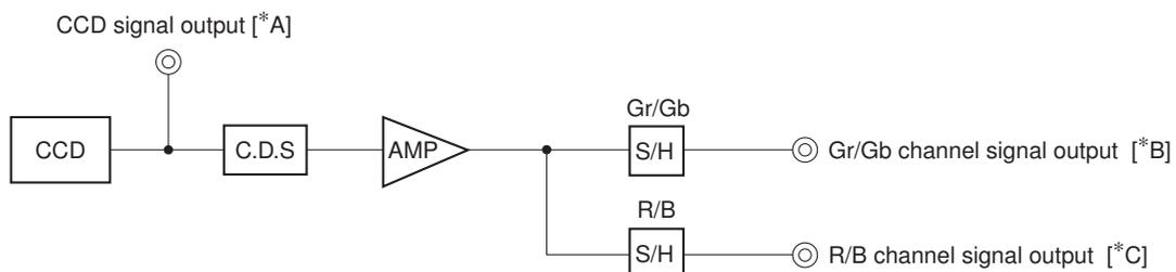
Note) Adjust the amplifier gain so that the gain between [\*A] and [\*B], and between [\*A] and [\*C] equals 1.
