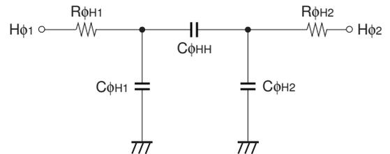
**Horizontal transfer clock equivalent circuit**
