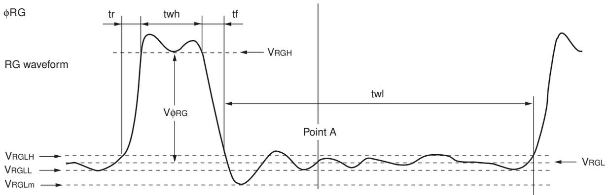
V<sub>RGLH</sub> is the maximum value and V<sub>RGLL</sub> is the minimum value of the coupling waveform during the period from Point A in the above diagram until the rising edge of RG. In addition, V<sub>RGL</sub> is the average value of V<sub>RGLH</sub> and V<sub>RGLL</sub>.
