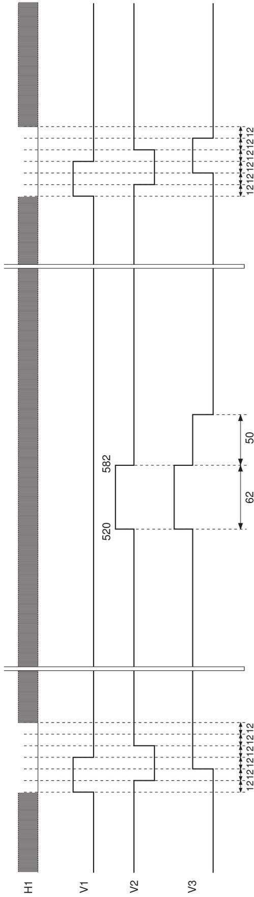
Drive Timing Chart (Horizontal Sync) Progressive Scan Mode
