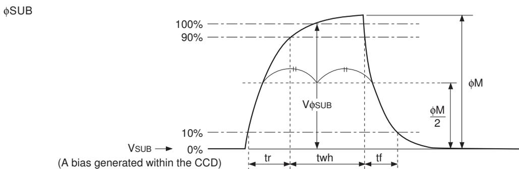
**Clock Switching Characteristics** (Horizontal drive frequency: 24.54MHz)
