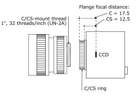
Fig. 3: The C-mount thread.
