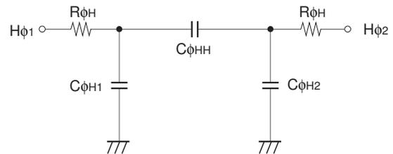
**Horizontal transfer clock equivalent circuit**
