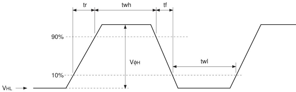
**(4) Reset gate clock waveform**
