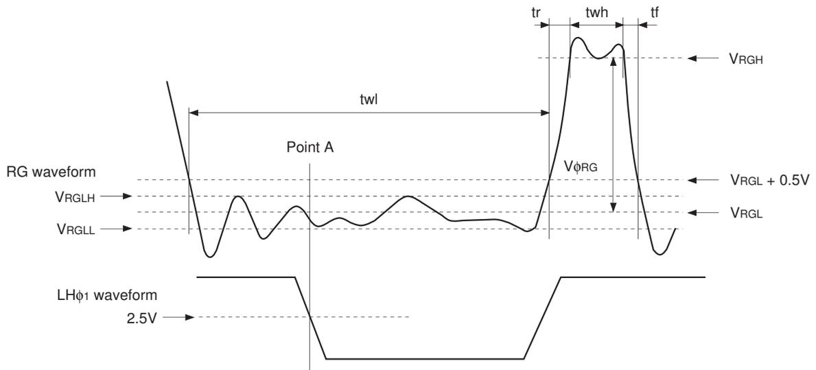
$V_{RGLH}$  is the maximum value and  $V_{RGLL}$  is the minimum value of the coupling waveform during the period from Point A in the above diagram until the rising edge of RG.
