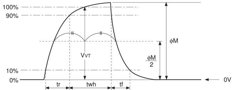
(2) Vertical transfer clock waveform
