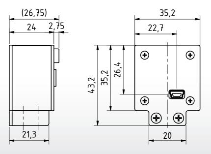
Dimensions: mm Tolerances: DIN ISO 2768m
